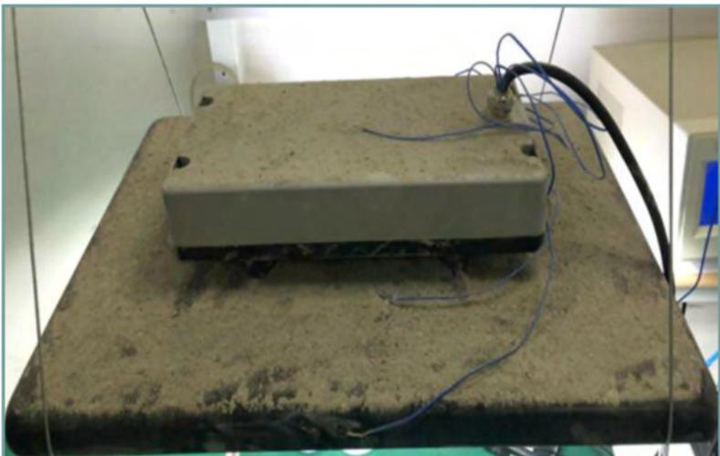
Exclusive dust testing, a simulation of 5 years of dust collection, resulted in a 2 degrees Celsius income of the Tc temperature on leds and driver.
