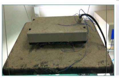
Exclusive dust testing, a simulation of 5 years of dust collection, resulted in a 2 degrees Celsius income of the Tc temperature on leds and driver.
